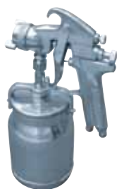
M1266 Air Pressure 45-70 PSI Air Consumption 8.0. C.F.M. - 12 C.F.M. Compressor required 1 1/2 Hp Air Inlet 1/4" PS (M) Fluid Inlet 3/8" PS (M) Capacity of cup 1 Litre Tip of Nozzle Ø 1,7 mm
